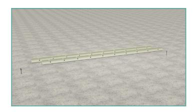
Position rails and connect together with either Compressible Rubber Cord, Straight Coupler Ferrules, Top Cap, or Top extender as required – ensure all rails are butted tightly together.
