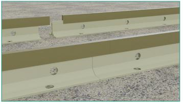
If extra height is required, place a pair of wedges under the rail base, close to where the pins are to be driven through, adjust to height required.
