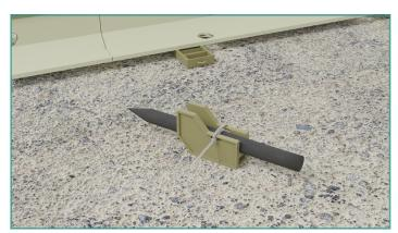
Position pins in holes on larger rails, or close to the rail base edge on the small rail, drive into sub base to desired depth.
